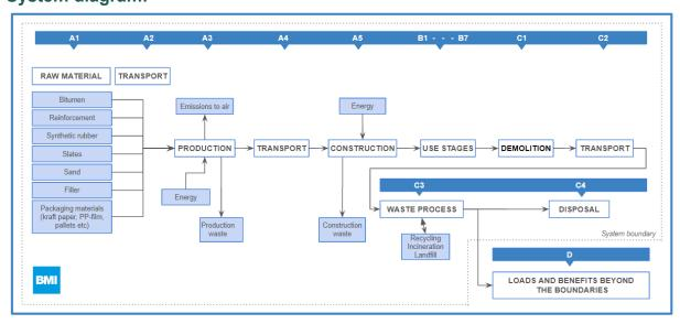
This is a Cradle to gate with options, modules C1-C4 and module D LCA. The life cycle stages included are as shown below (X = module included, ND = module not declared).
